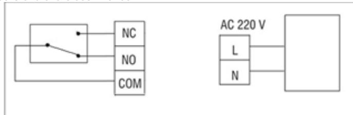
CONNECTION EXAMPLES WITH GAS BOILER SYSTEMS- THERMOSTAT PNI CT400 \*
