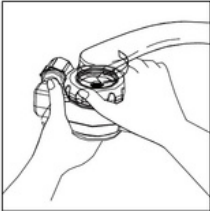
4. Tighten the connecting nut and fix the main body
